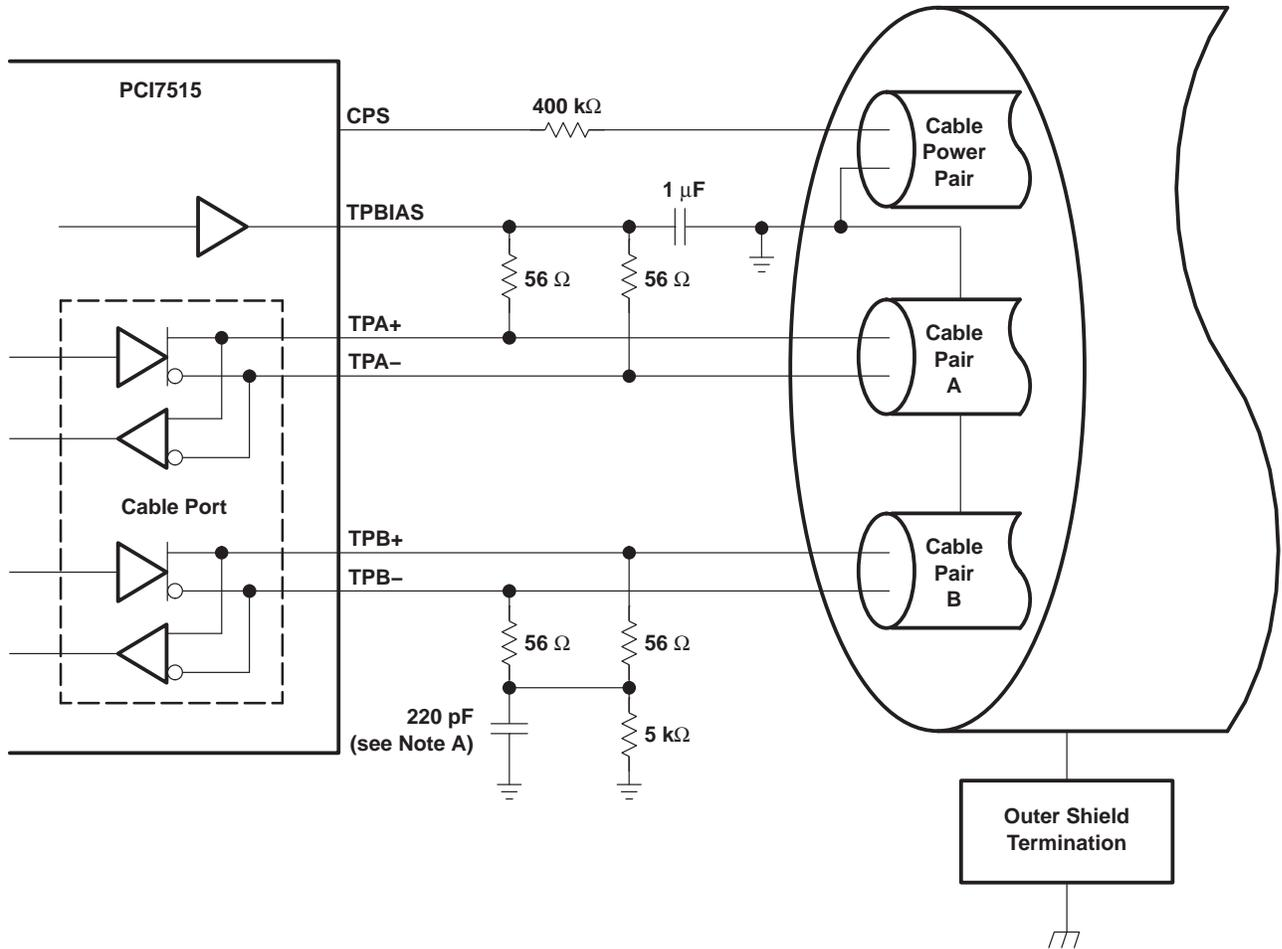
NOTE A: IEEE Std 1394-1995 calls for a 250-pF capacitor, which is a nonstandard component value. A 220-pF capacitor is recommended.
