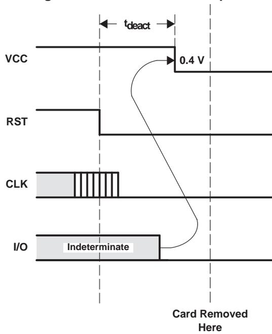
Figure 12-4. Contact Deactivation Sequence
