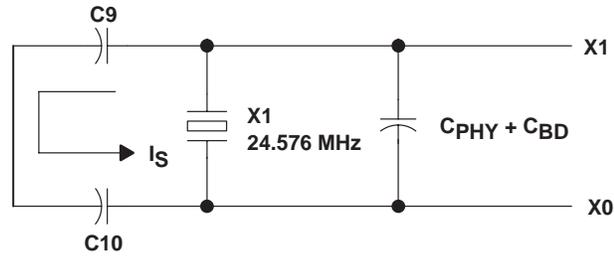
**Figure 3-19. Load Capacitance for the PCI7515 PHY**
